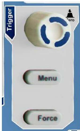
Trigger control panel
